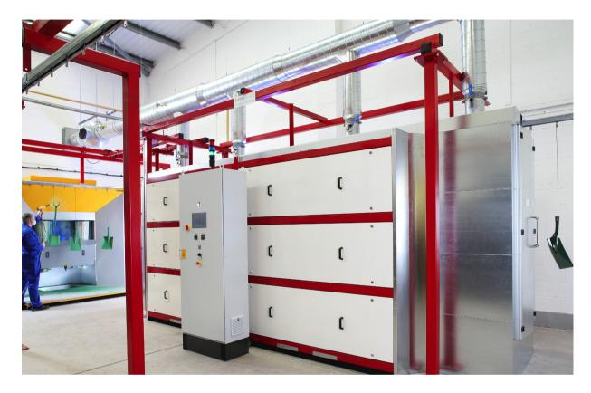
Infrared heat transfers energy and generates heat where it is needed. PLC controlled gas catalytical infrared ovens are precisely designed to match the thermal process application. This saves energy, improves process stability and increases capacity and quality. With our Application Center we offer all our customers the opportunity to answer important questions, from a practical viewpoint. Competent, technically experienced employees carry out and monitor the tests.
